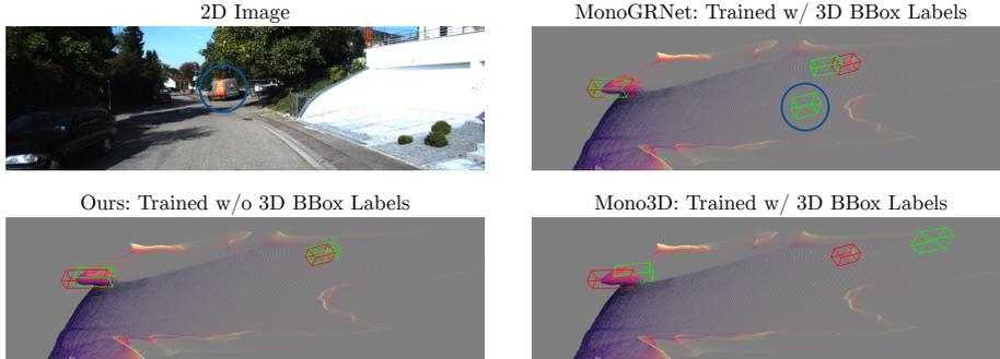
**Fig. 1.** Qualitative comparison of Mono3D [1], MonoGRNet [6], and Ours. We show ground truth bounding boxes for cars (*red*), predicted bounding boxes (*green*), and the back-projected depth map from BTS [5]. The proposed model can deliver comparable qualitative results to MonoGRNet. Note that the extra prediction from MonoGRNet (*blue circles*) is not a false positive because it corresponds to a van, which is not a false positive in KITTI.
