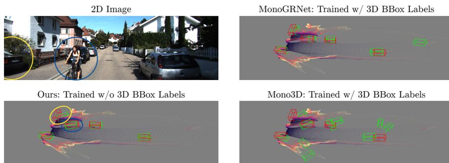
(a) Our model is able to predict the position and orientation of the car occluded by the cyclist (*blue ellipses*) without training with 3D bounding box labels. However, it still struggles with the heavily truncated car on the left, but still delivers a better prediction than Mono3D (*yellow ellipses*).
