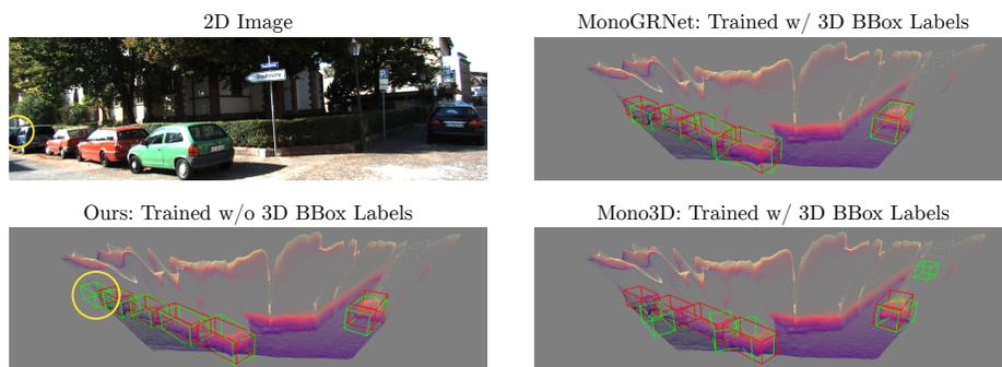
(b) Our model predicts an additional car (*yellow circles*) because it is slightly visible on the 2D image and detected by Mask R-CNN. The image shows that the proposed algorithm can handle vehicles with mild occlusion well.
